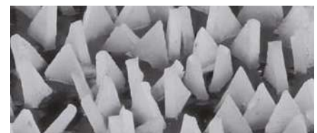
The VICTOGRAIN abrasive grain is optimally aligned
