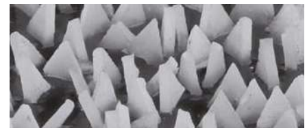
The VICTOGRAIN abrasive grain is optimally aligned
